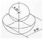
a) The isometric projection of a sphere is a circle whose diameter is equal to the isometric diameter of the sphere.
